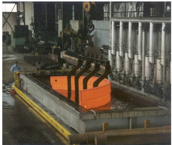
Exhibit 4: Forged Half Rings being polymer quenched
