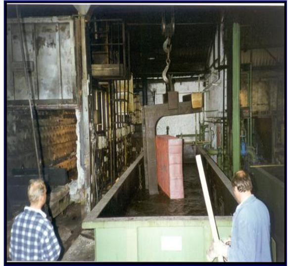
Exhibit 2: Tool Steel Block being polymer quenched
