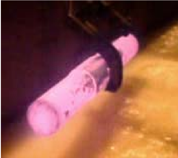
Exhibit 1: Alloy Steel Turbine Shaft being polymer quenched
