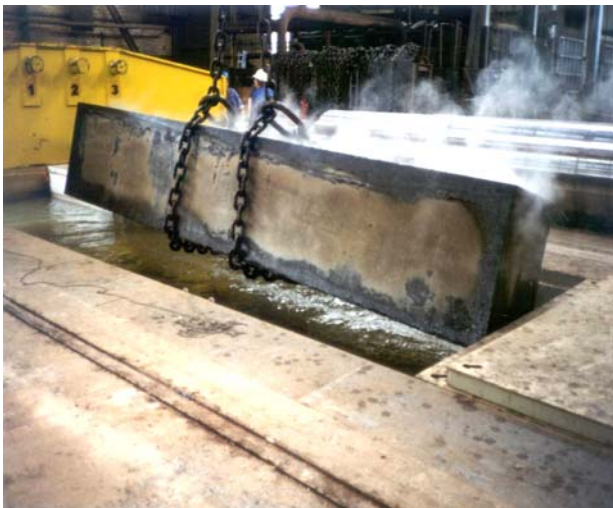
Exhibit 3: Tool Steel Block after quenching in polymer quenched
