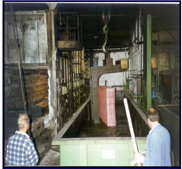
Exhibit 2: Tool Steel Block being polymer quenched
