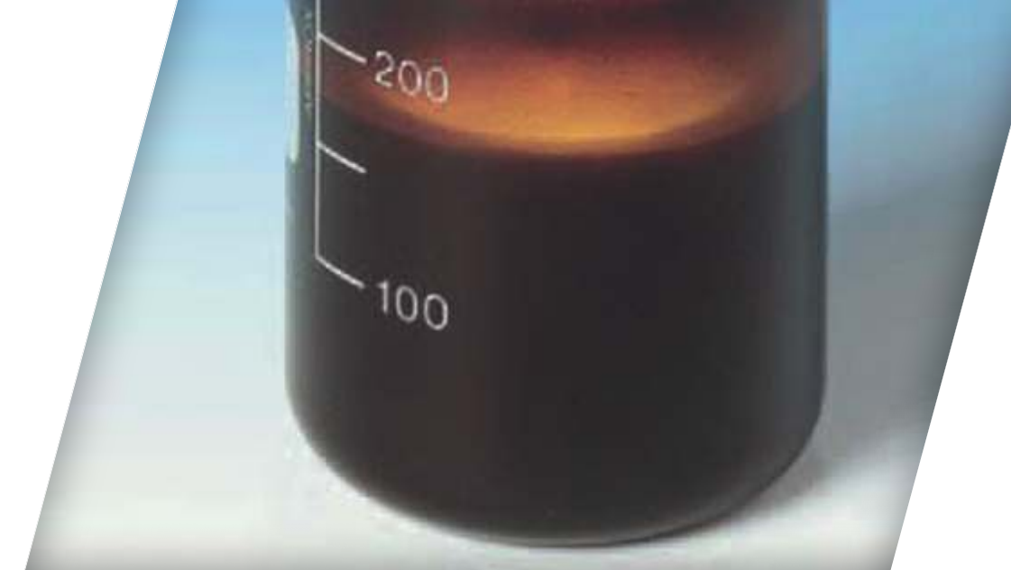
Quenching oil with poor ageing resistance after an oxidation test.
