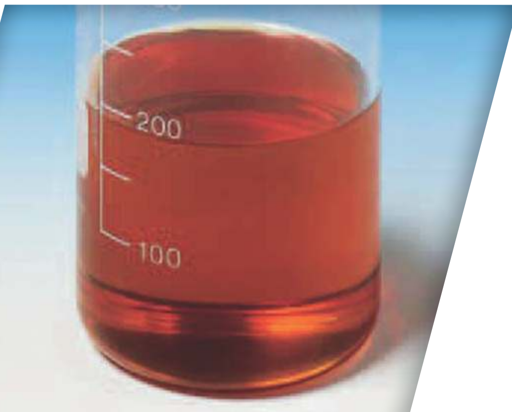
Quenching oil with good ageing resistance after an oxidation ageing test.
