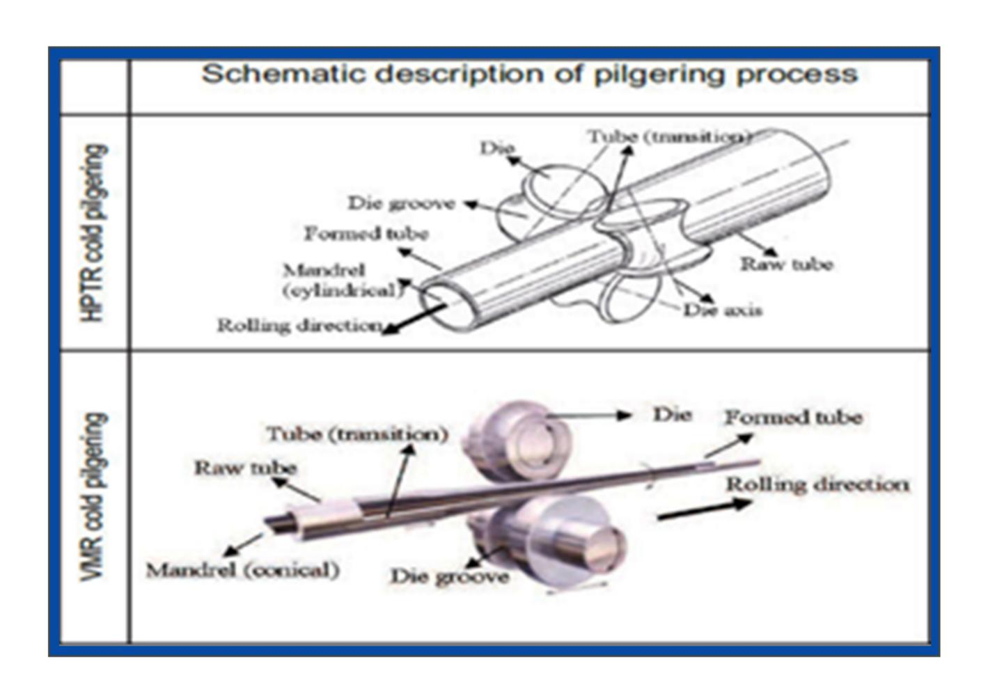
The basic idea of this method is to reduce both the diameter and the wall thickness of the tube and improving the grain structure of the material. The tube wall thickness is reduced and simultaneously it becomes elongated. The elongation contributes to the productivity of the method and is directly related to the amount of area reduction applied. This depends on the mandrel and roll die design and motions.
