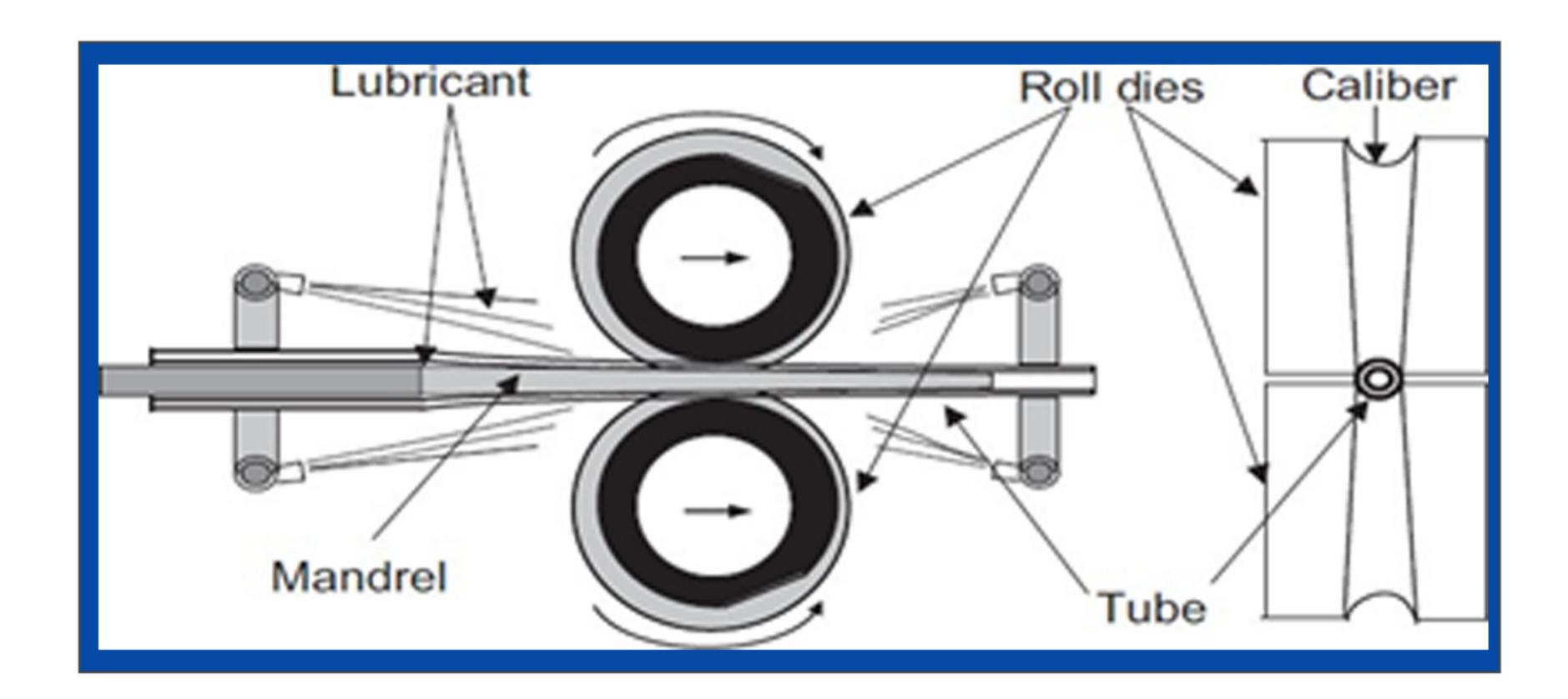
Lubrication is a key factor in the cold pilgering operation in terms of productivity as in most metal forming operations. This is due to several reasons.
