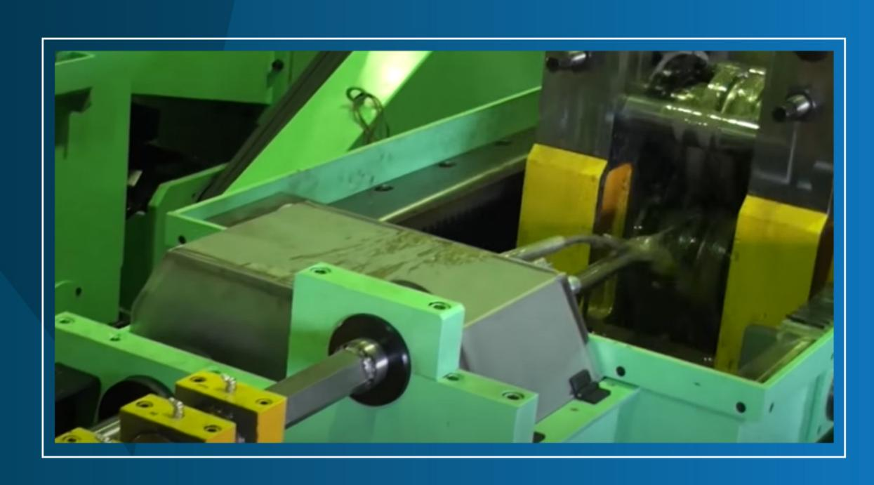
Cold pilgering is one of the two major method used in seamless tube production. Other major method is cold drawing but cold pilgering has several advantages that are:-
